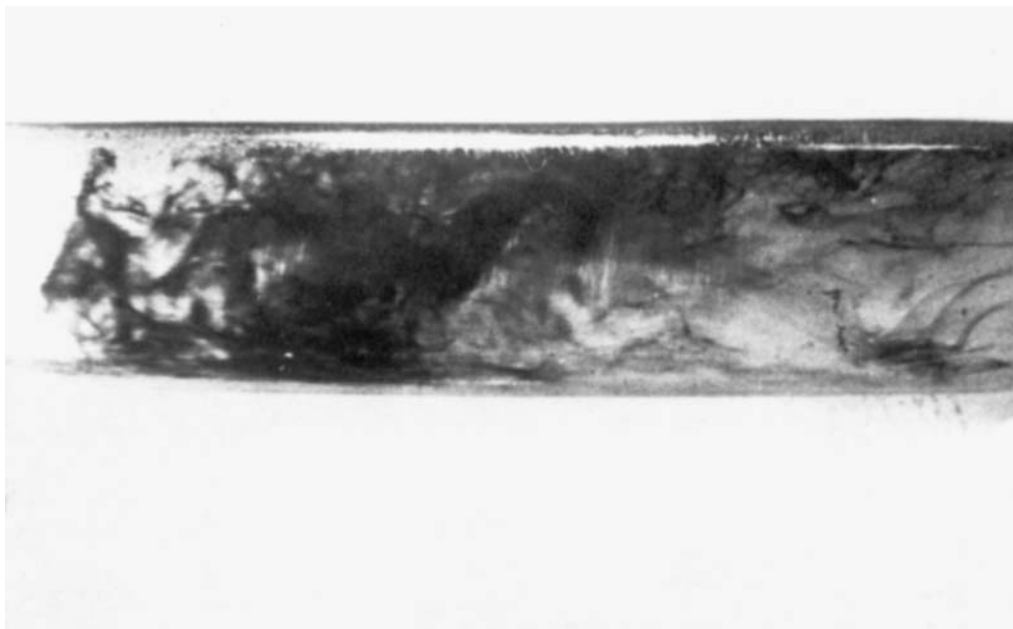
FIGURE 1. A view through a transparent section of the pipe showing the dye pulse at less than 1 m from the injection device.
